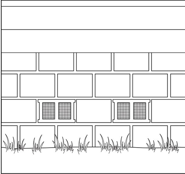
Figure 20. Concrete block turned sideways (insect screening shown)
